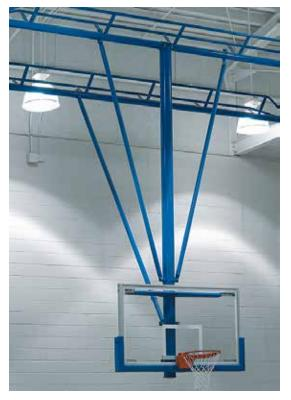
■ For spaces where folded backstops are not required, the ceiling-braced, stationary TS-21 Basketball Backstop offers flexible installation. Ceiling-suspended and rear- or front-braced to allow backstop to be used in many building conditions. Backstops are custom designed so the lateral sway brace intersects the main mast at approximately 54" (1.37 m) above the goal and 18" (46 cm) above the backboard; to ensure maximum rigidity.
